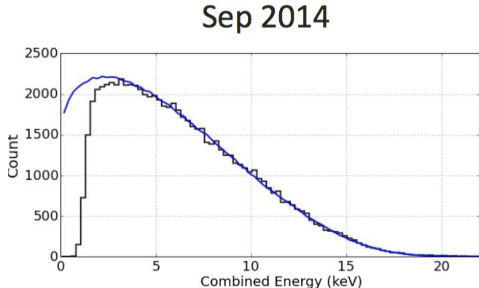
libNEST tritium reconstructed energy spectrum is a better representation of data when the box cut is made
