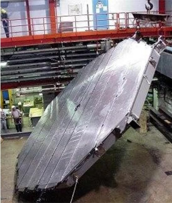
484 planes of steel mounted with scintillator strips totaling 5.4kT.
