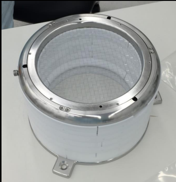
Reverse Field Region of the TPC with the Cathode Grid mounted
