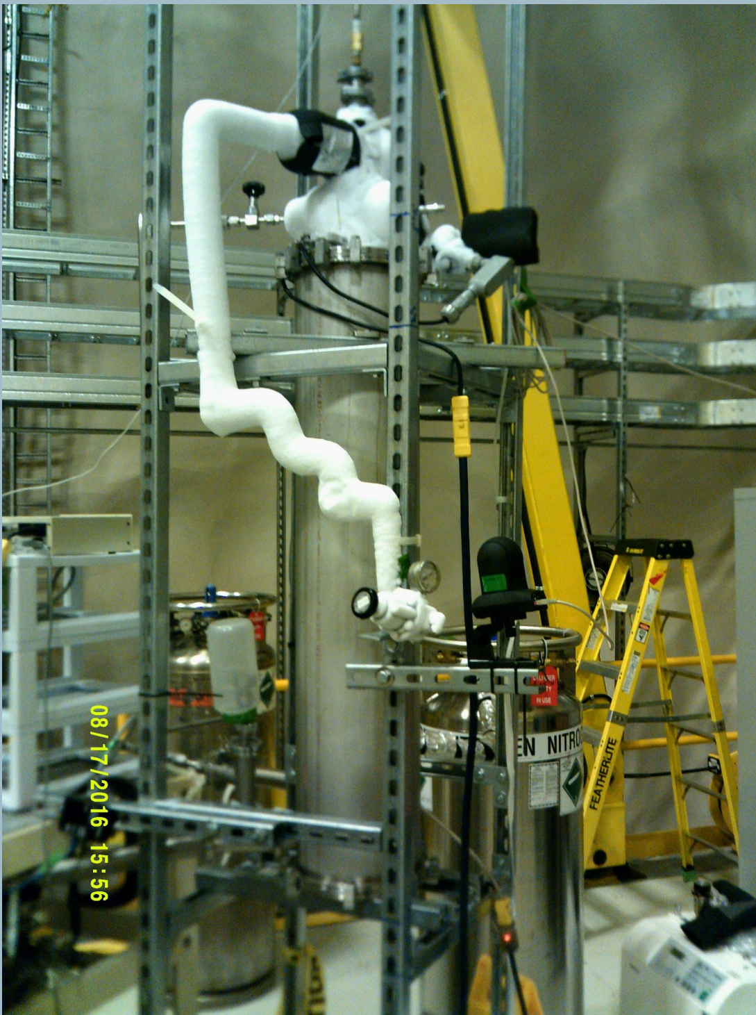
Figure 4. The condenser while in operation, which utilizes liquid nitrogen, at 77 K, to cool down the argon to its liquid form below 87 K.
