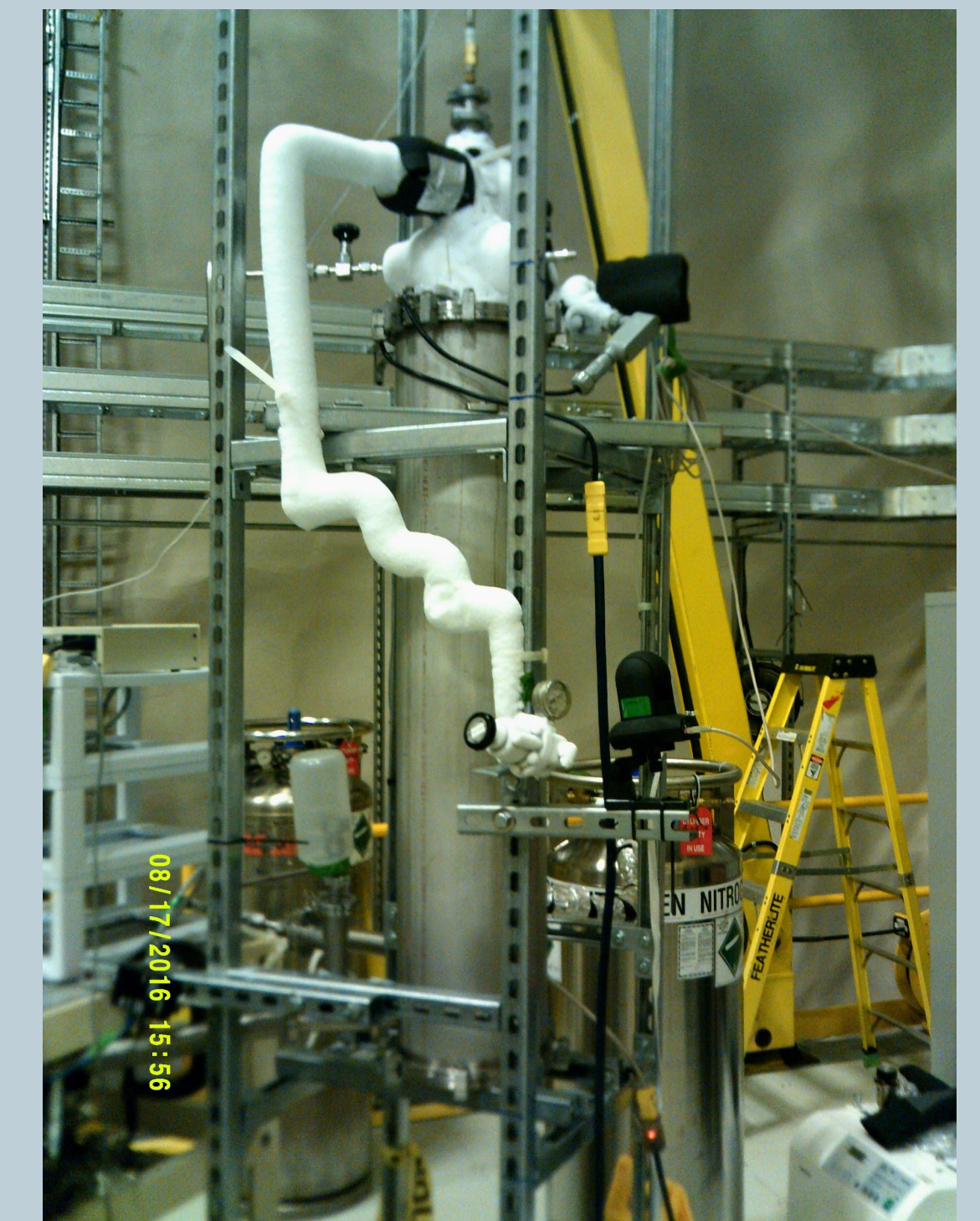
Figure 4. The condenser while in operation, which utilizes liquid nitrogen, at 77 K, to cool down the argon to its liquid form below 87 K.
