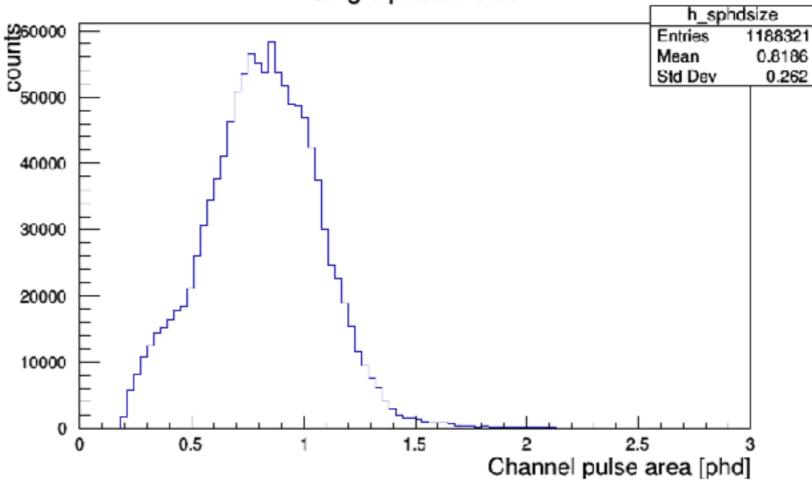
(above) Pulse area detected for pulses identified as single PE where only 1 PMT triggered for the pulse. The data is from the MDC1 July 20-23, 2017 datasets.
