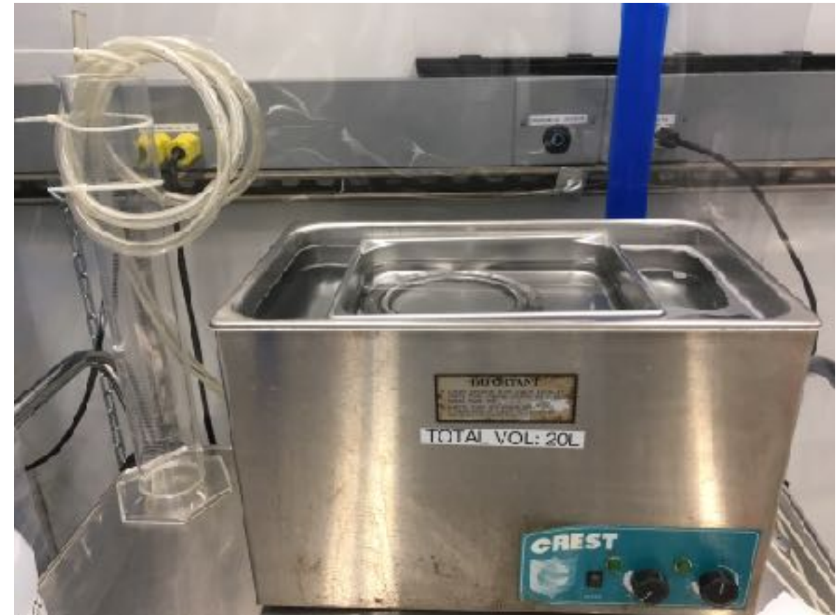
Figure: Anode grid is placed in a tray within the ultrasonic cleaner in the cleanroom. DI water added to the tray spills over into the main bath visibly removing some debris from the water surface. Grid is removed from the tray once the surface is visibly clear.
