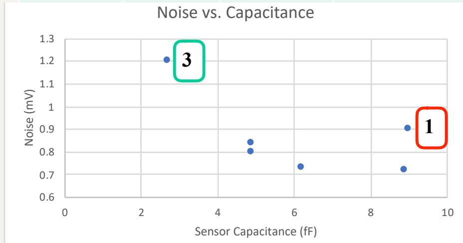
**Extra noise pick up appears to occur mainly through capacitive coupling to the sensor**
