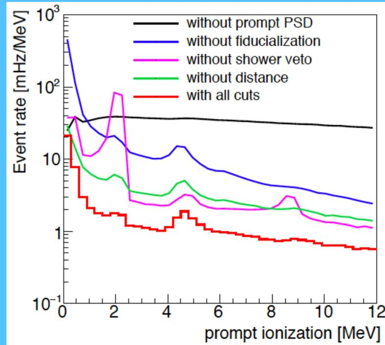
The muon simulation with PROSPECT. In the near surface situation, muons produce less correlated background than cosmogenic neutrons.
