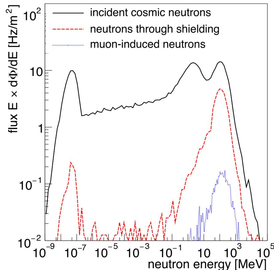
Ambient surface neutron spectrum, and toy model processed through 1 m.w.e. shielding.
