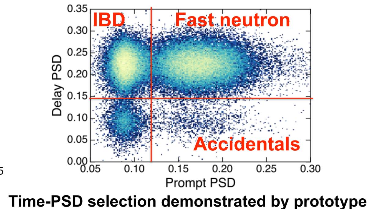
Time-PSD selection demonstrated by prototype
