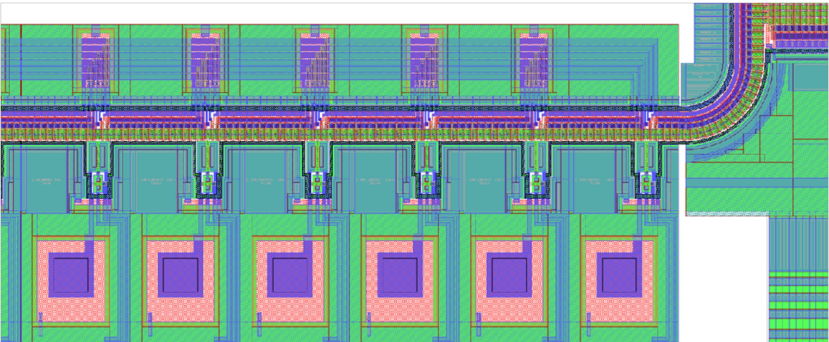
**R&D: 6x Multiplexing in Readout Structures**
