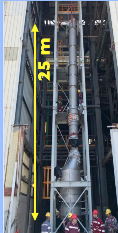
Seruci 0 – prototype Column tested
