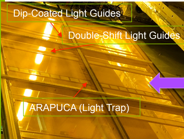
58 light guide and 2 ARAPUCA photon collectors
