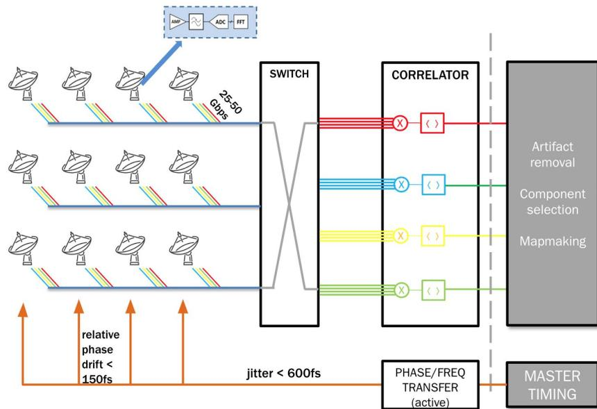
*Jitter, phase calibration and stability of the clock distribution are critical.*
