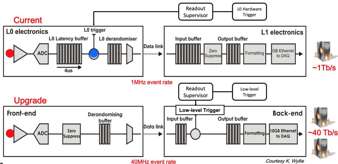
Triggerless readout, which can read out 40 MHz
