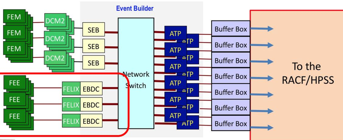
Hybrid with triggered calorimeters
