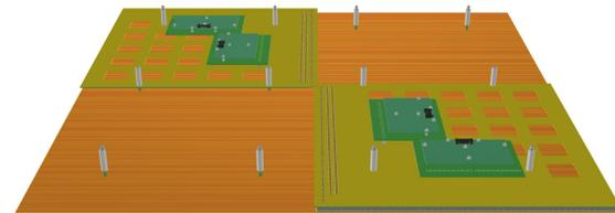
Integrating the FE electronics (FEMB of ProtoDUNE) on the PCB
