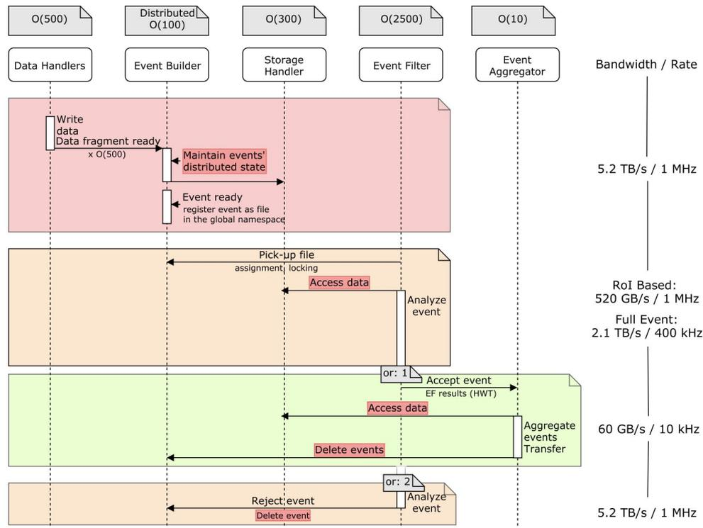
Logical communications between different components of the Dataflow system
