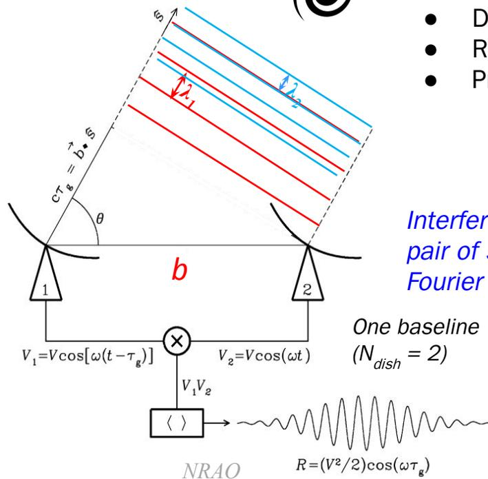
*Interferometer measures the sky image directly in the Fourier space. Every pair of stations provides a baseline, measure a 'Visibility', which is a Fourier component of the image.*
