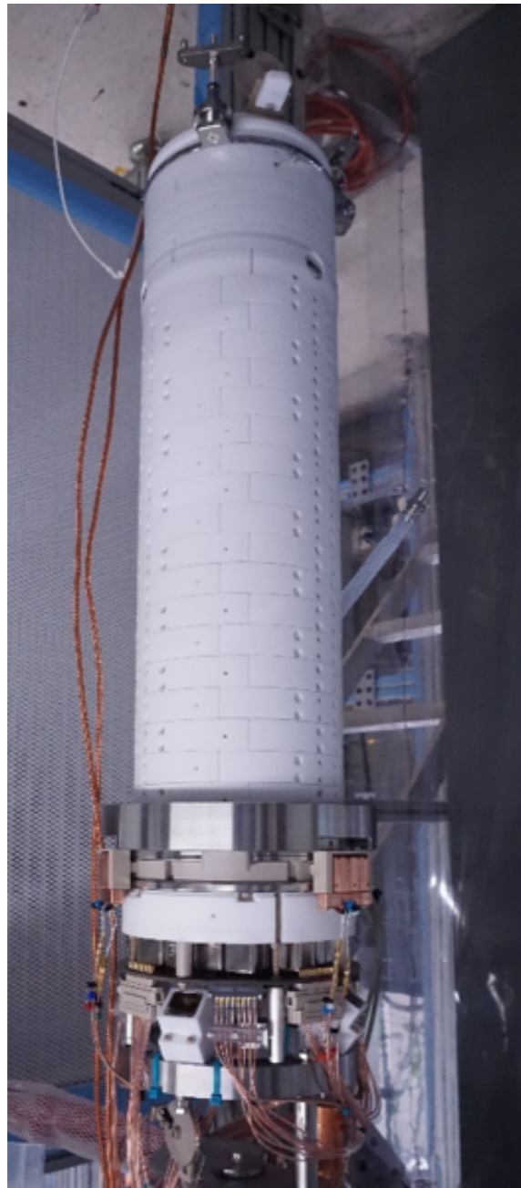
Designed as TPC to test cryogenics, circulation, HV
