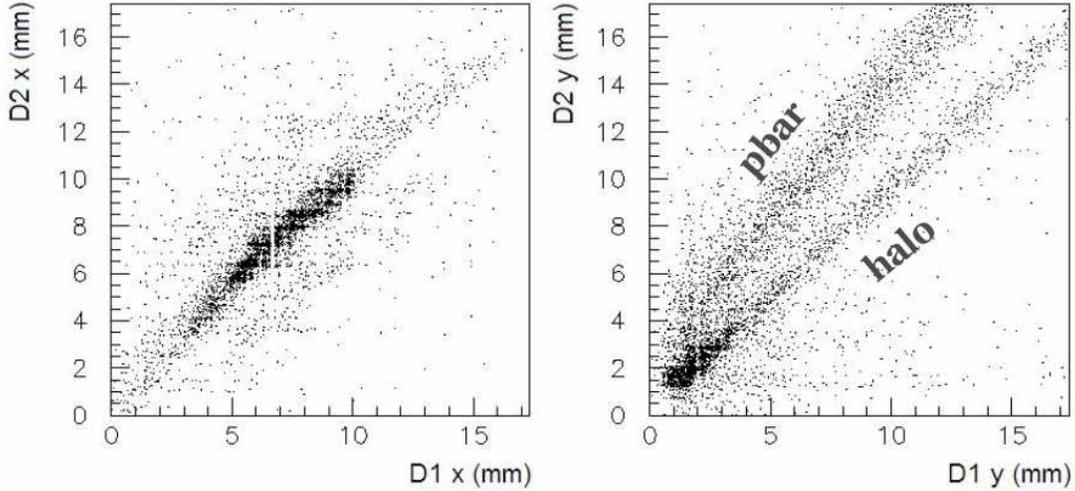
**FIGURE 3.** Hit correlation for the dipole spectrometer. On the left, the x coordinate of a hit on the first detector is plotted against the one on the second detector; on the right, the same correlation is plotted for the Y coordinate
