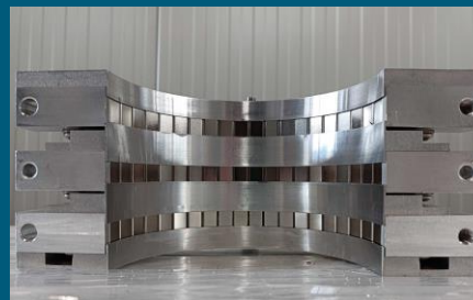
Alternate polarity permanent neodymium bar magnets
