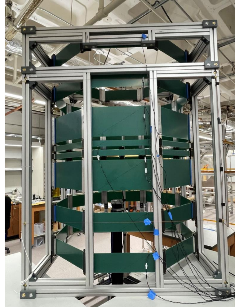
Half-scale model of B0 coils
