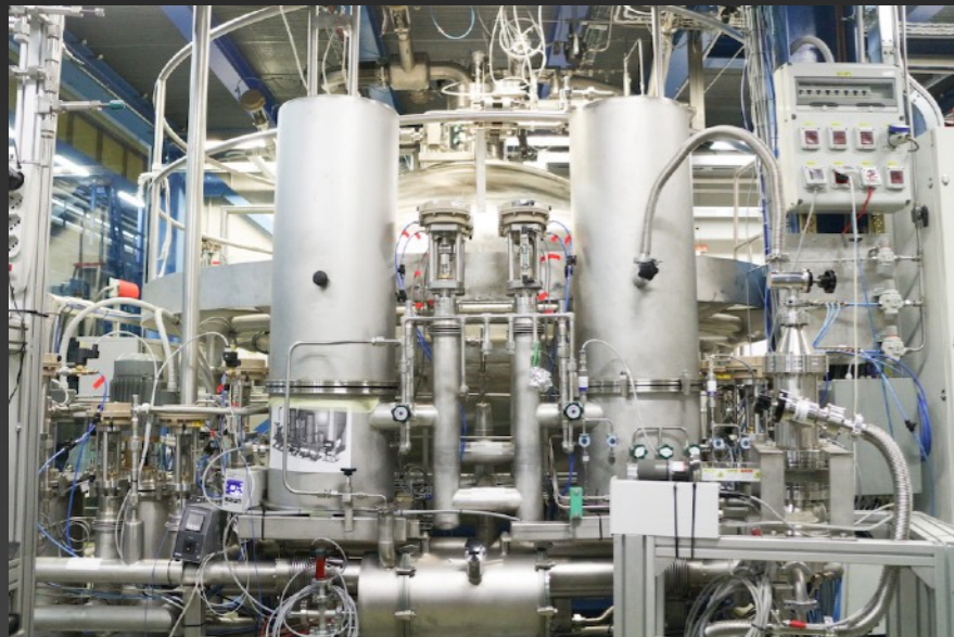
Liquid purification system
