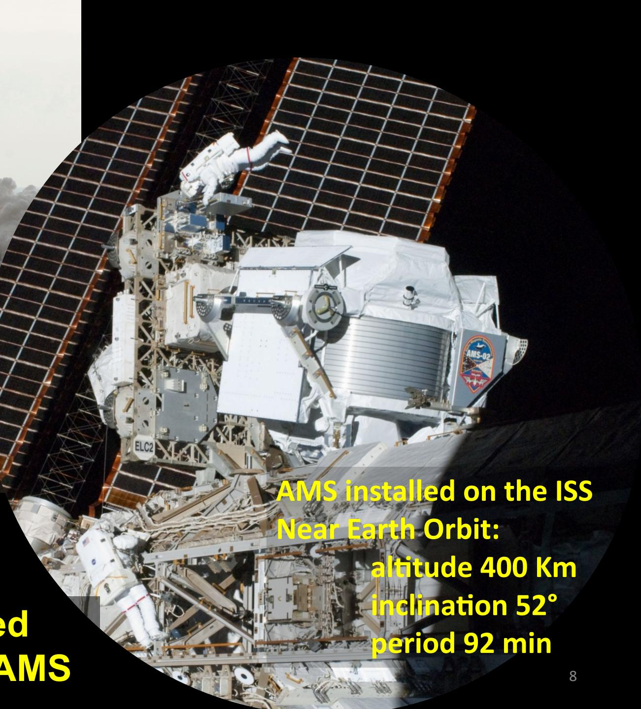
AMS installed on the ISS
