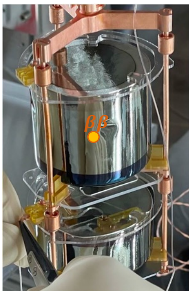
Ge detector with PEN plate holders
