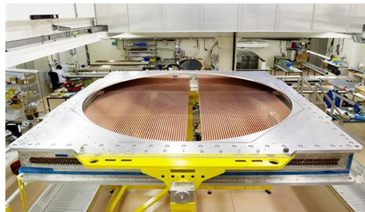
A current NA62 STRAW chamber
