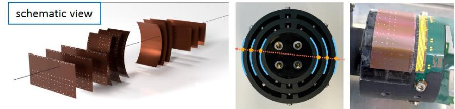
Full-size prototype of half-layers (unprocessed silicon)
