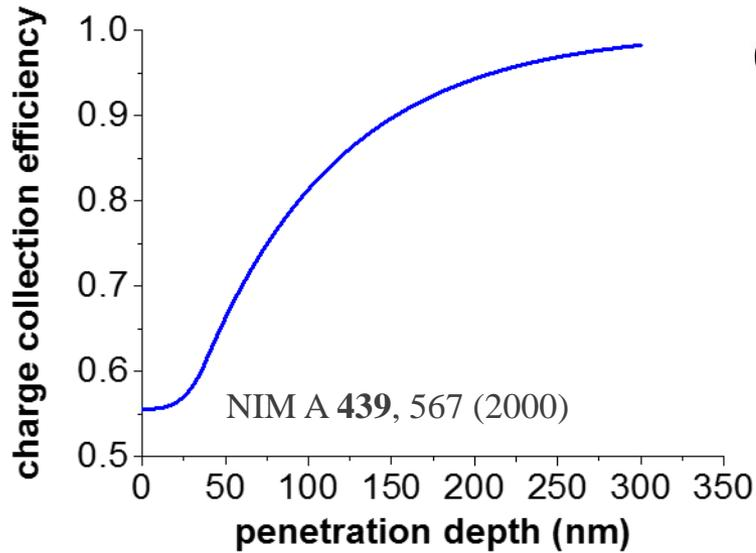
Charge collection efficiency in active layer of similar detector (Simulation with SRIM)
