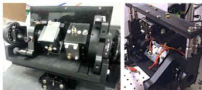
Left: RTP pockels cell in its mount. Right: An example of helicity patterns like those used for PREX-II.
