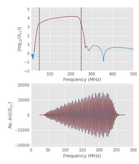
Measured from HERA Phase II amplifier electronics
