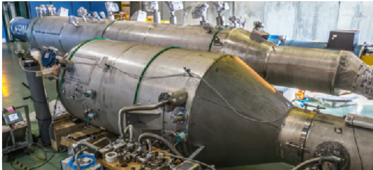
Part of DS-20k distillation column
