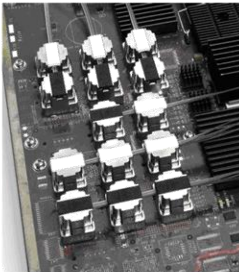
Figure 2. MiniPOD™ Transmitter and Receiver flat ribbon cable modules in a tiled arrangement example.
