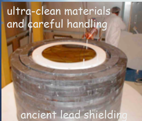
Passive shielding: Pb shielding
