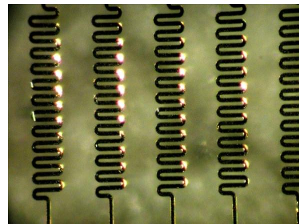
After etching of Si wafer
