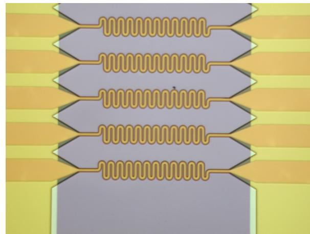
Before etching of Si wafer
