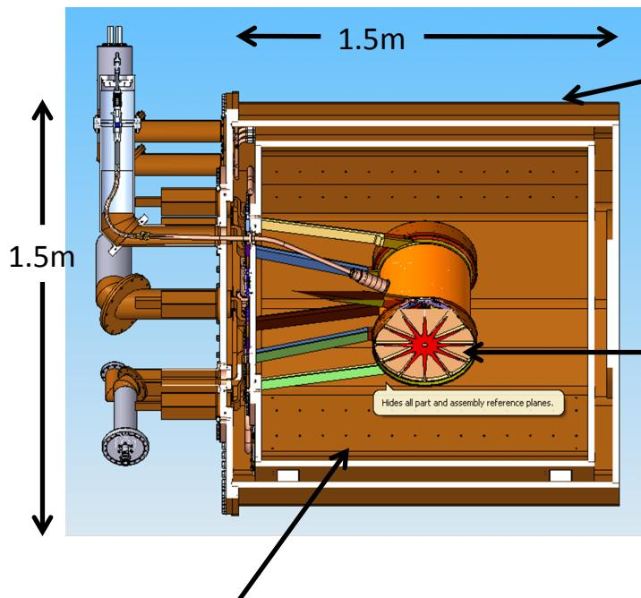
Inner cryostat filled with 50 cm HFE7000 cooling/shielding fluid ( $\sim 1.8 \text{ g/cm}^3$  at 170 K)
