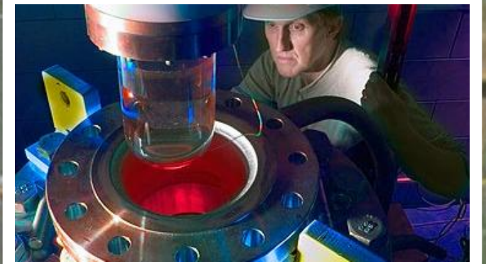
COUPP (2 kg / 1 liter) Room temp \text{CF}_3\text{I} Bubble Chamber
