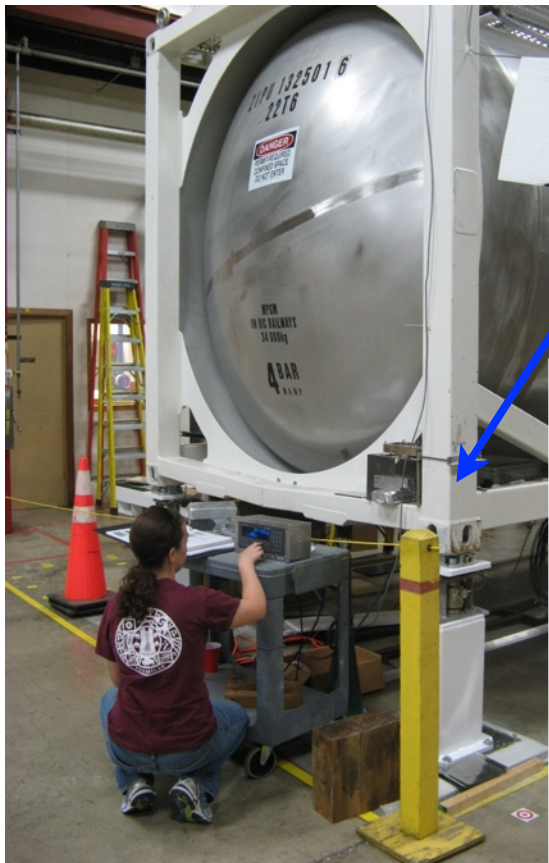
ISO weighing tank and load cells
