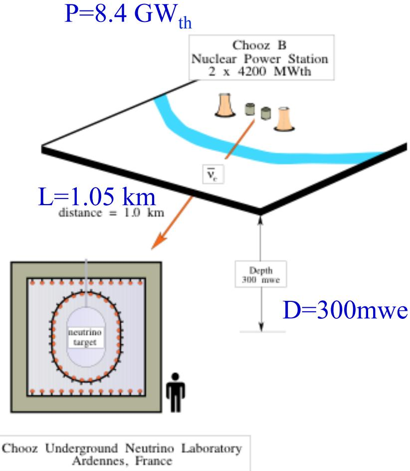
m = 5 tons, Gd-loaded liquid scintillator
