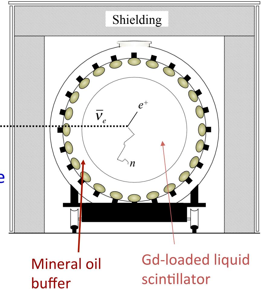
Events selected based on coincidence of  $e^+$  signal ( $E_{\text{vis}} > 0.5$  MeV) and  $\gamma$ s released from  $n + \text{Gd}$  capture ( $E_{\text{vis}} > 6$  MeV).
