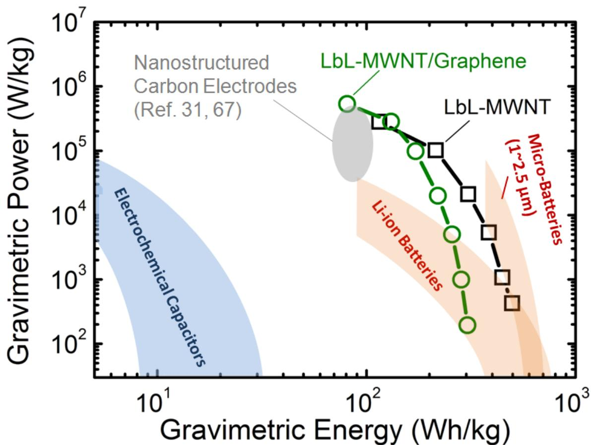
5-10x increase in power relative to Li-ion batteries
