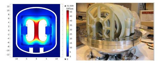
**Figure 6.** Rogowski electrodes for the MSHV system of the SNS nEDM experiment. (left) FEM calculation of the electric field inside the CV showing a uniform field in the gap. (right) A photograph of the Rogowski electrodes installed in the CV.
