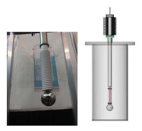
**Figure 18.** New test stand for liquid argon breakdown measurements at the LHEP Bern using a maximum electric field of 1.2 MV/cm, a maximum voltage difference of 130 kVcm, and a distance range of 1 mm up to 10 cm measured with 100 microns accuracy.
