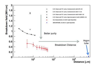
**Figure 17.** Literature versus recent measurements of high voltage breakdowns in liquid argon at LHEP Bern. The higher the argon purity, the lower the breakdown field. The effect on the cathode ground distance needs to be studied further.
