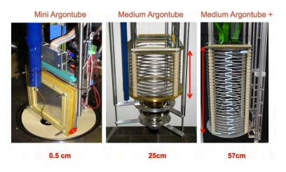
**Figure 12.** Liquid argon TPC evolution at LHEP Bern. From very short drift of 0.5 cm distance TPCs the drift distance increased in size to a 25 cm drift TPC equipped with a Hamamatsu PMT, and a 57 cm version for UV laser ionization measurements.
