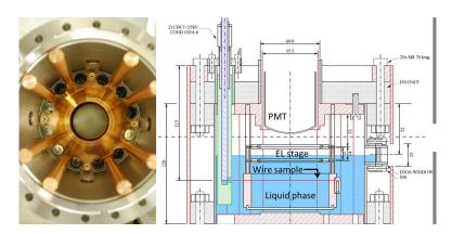
**Figure 36.** Left: Interior of the cathode wire test chamber at Imperial College London for LZ R&D purposes. The upper part is shown with the PMT, available ports, copper structure for heat distribution and 4 viewports. Right: A sketch of the chamber.
