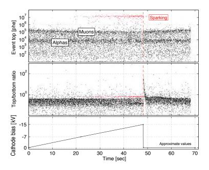
**Figure 28.** Event area, top/bottom ratio and C grid bias as a function of time during one of the LUX high voltage bias trials in liquid xenon at the surface laboratory. For this trial, light production at the  $10^7$  phe level appeared at about -7 kV and electric breakdown took place at -15 kV.
