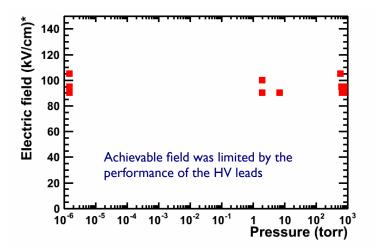
**Figure 7.** Electric field strength achieved in liquid helium for a 1 cm gap between two electropolished stainless steel electrodes 12 cm in diameter. Note that the achievable field was limited by the performance of the high voltage leads. The hydrolic pressure of liquid helium is  $\sim 0.1$  torr/cm
