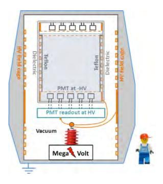
Figure 1. Possible design for a large dielectric cryostat.
