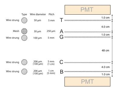
**Figure 27.** The LUX electrostatic grid configuration: top (T), anode (A), gate (G), cathode (C) and bottom (B) grids. All grids are made from stainless steel wire. For C and B, the pitch and diameter values used during surface operations are shown in parenthesis.
