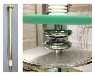
**Figure 23.** (left) Image of the GLACIER test apparatus high voltage feed-through. (right) The electrodes structure.
