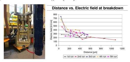
**Figure 16.** Breakdown measurements in liquid argon at the LHEP Bern using a maximum electric field of 30 kV and a maximum distance of 1 cm distance measured with micrometric precision.
