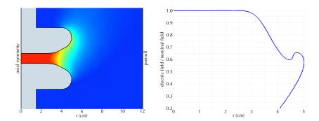
**Figure 24.** (left) Computed electric field for GLACIER test electrodes. The cross sections of the electrodes are shown in grey, and the color pattern is proportional to the absolute value of the electric field. The electric field is essentially uniform in the central region. (right) Computed electric field on the profile of the top electrode as a function of the radius. The largest field is attained between the electrodes.
