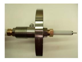
Figure 38. The NEXT-DEMO high-voltage feed-through, designed and built by Texas A&M
