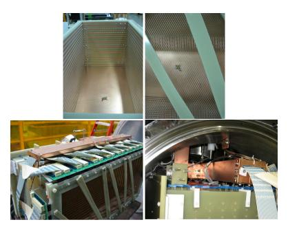
**Figure 9.** Looking into the ArgoNeuT liquid argon TPC field cage before (top left) and after (top right) installation of the wire planes. The ArgoNeuT TPC before (bottom left) and after (bottom right) installation in the cryostat.
