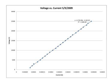
Figure 11. Current-Voltage curve for ArgoNeuT liquid argon TPC.
