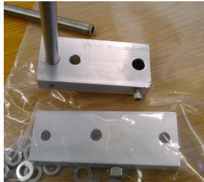
Below: Aluminum blocks for mouning instruments and PMT.
