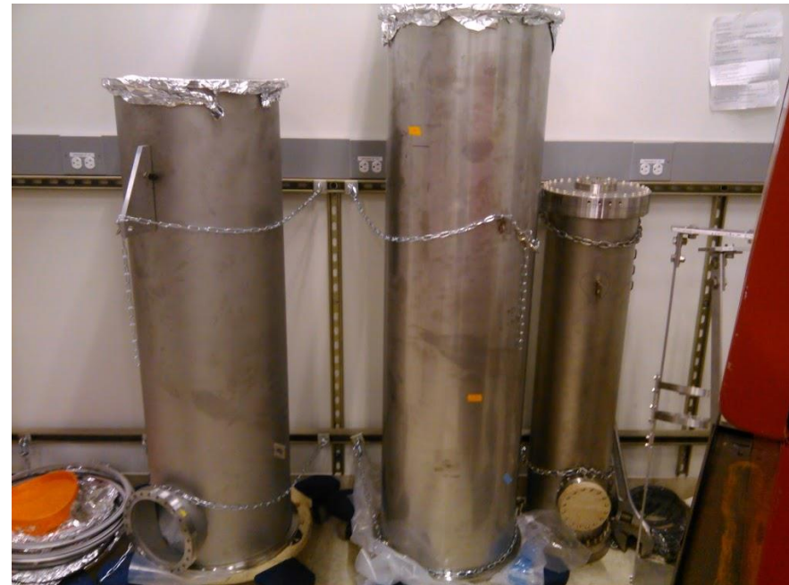
Leftmost: R&D Vacuum vessel. Middle: Purification tower vessel. Right: R&D Xenon Vessel.
