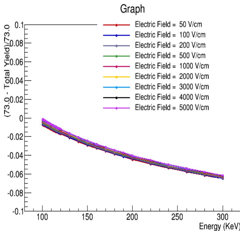
Plot shows the total yield variation wrt to 73 for nuclear recoil as a function of energy for different electric fields.
